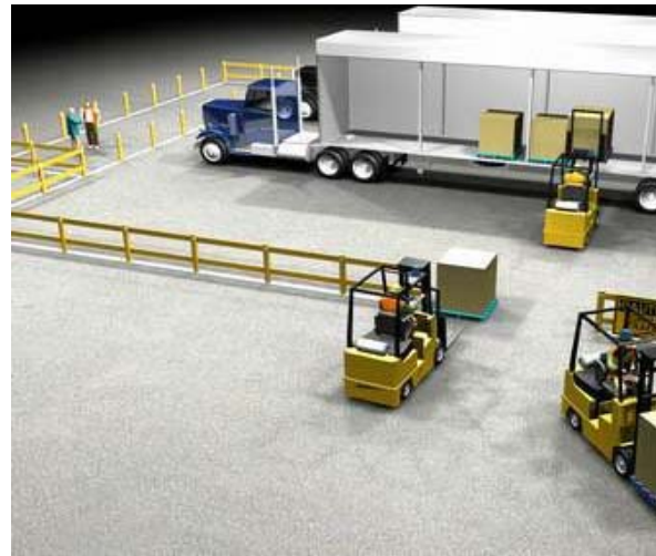
Loading/receiving area with truck drivers physically separated from forklifts
